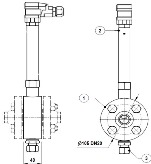
Remarks: Can be fitted into a "T" connection or into our standard chamber, providing that the probe is always in contact with the water. Any metallic parts near the probe must be at a minimum of 20 mm of distance from the central end pole.
