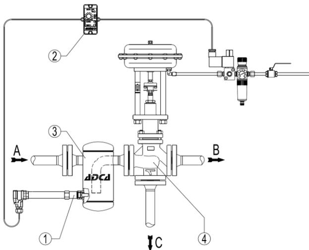
**WATER TUBE COIL BOILER – PROBE INSTALLED IN THE RECIRCULATING PIPE**
